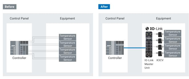
Reduces wiring between control panels and equipment
