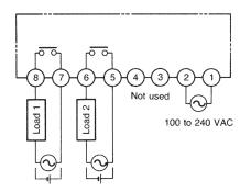
Note: To each load, connect the power supply for load.
