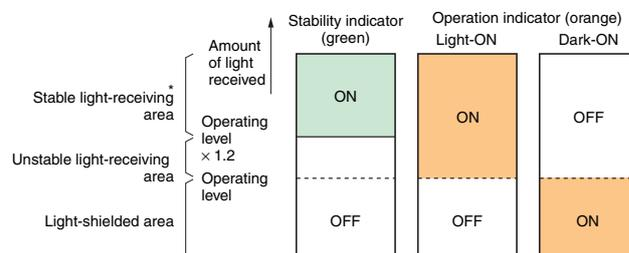
\* If the Receiver is set to the stable light-receiving area, it will become more resistant to environmental fluctuations such as temperature, voltage, dust, and setting deviation after installation. For applications where a stable light-receiving area is not obtained, attention must be paid to environmental fluctuations.
