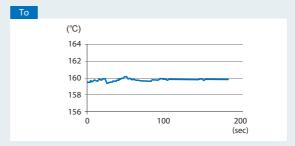
When the automatic filter adjustment function of the E5 $\square$ D /NX-TC is used, this periodic temperature variation is suppressed automatically. It becomes possible to perform stable temperature control.
