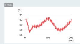
When a temperature sensor for a packaging machines is used, there is sometimes periodic temperature variation generated when there is a marked effect from the heat on the packaging materials side.
