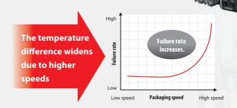
The temperature of the sealing surface is stably controlled automatically with measurement of the sealing surface temperature and algorithms to suppress variations.
