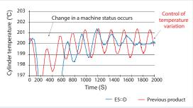
\* Data measured by OMRON on a water-cooled twin screw extrusion molding machine.
