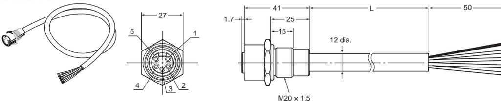
Note: A rubber seal and nut for panel mounting are included.
