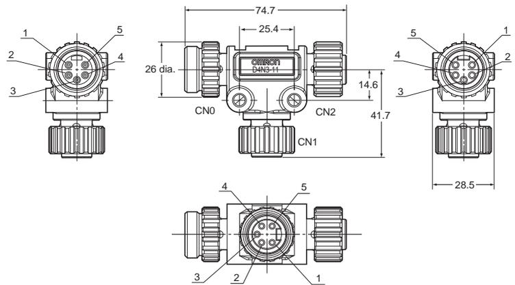
**T-branch Connector (5 Conductors for Communications,
