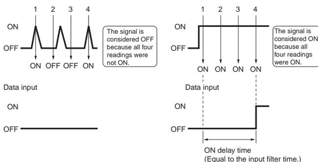
● **Function to Prevent Incorrect Inputs Caused by Inrush Current when Power Is Turned ON (input only)**
