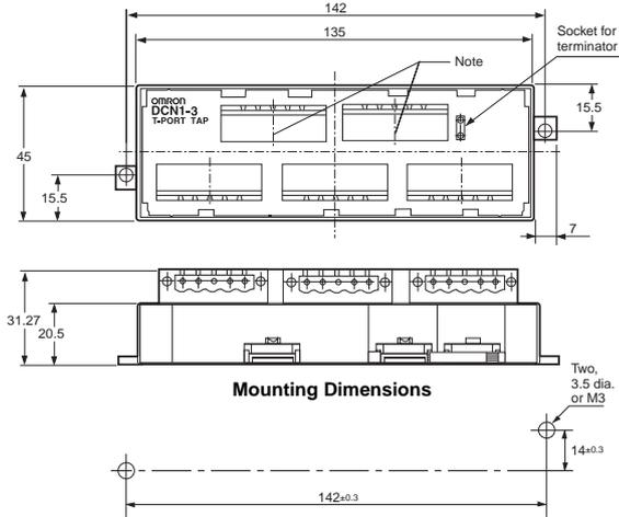
**Note:** When connecting a branch line to the main line, connect the main line to the connector marked with an asterisk because the resistance between the asterisked portion is minimal.
