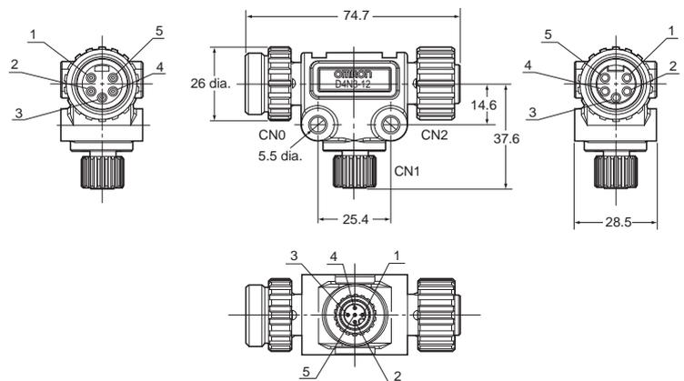
**Connector (Plug) with Terminating Resistance
