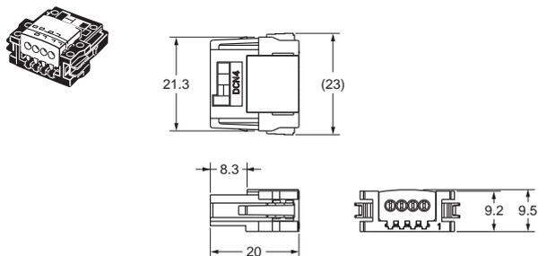
**Power Supply Terminal Block with Terminating Resistance for Flat Cable
