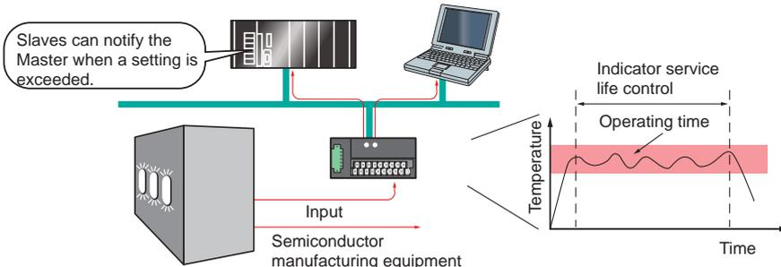
The peaks or valleys of temperature inputs that change in a regular pattern are counted to predict when devices operating with severe temperature swings are due for maintenance.
