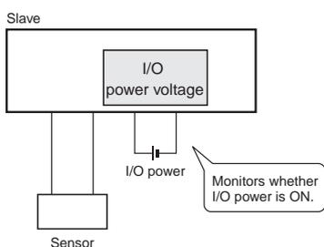
● **Sensor Power Short-circuit Detection Function (input only)**
