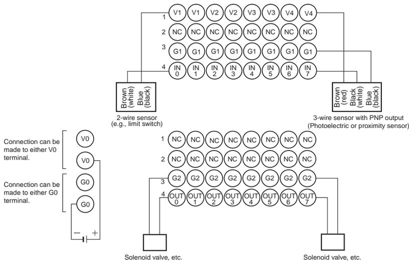
MIL Connector Terminals with Transistors
