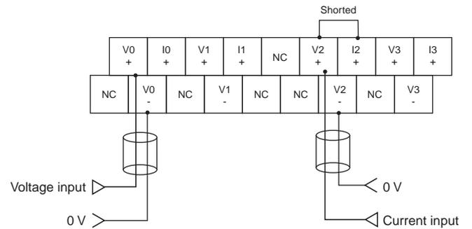
**Note:** With using a current input, always short the V+ and I+ terminals. (Use the shorting bar provided with the Unit.)
