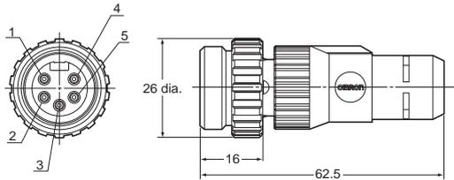
**Panel-mounting Connector (5 Pins for Communications)
