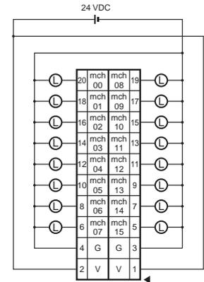
Wiring Diagram of Connector Cable Provided with the DRT2-ID16MLX(-1) and DRT2-OD16MLX(-1)
