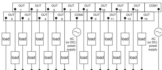
Transistor Remote I/O Terminals with 3-tier Terminal Blocks
