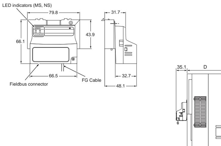
**Note:** After the DeviceNet™ Communication Unit is installed, dimension D of the inverter increases by 35.1 mm. (Dimension D of the inverter varies depending on the capacity. Refer to the RX-series V1 type USER'S MANUAL (Cat.No.I578))
