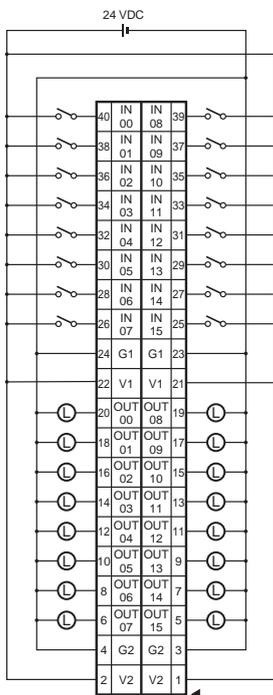
Screw-less Clamp Terminals with Transistors
