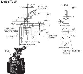
**Note:** Unless otherwise specified, a tolerance of ±0.4 mm applies to all dimensions.
