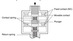
Conforms to EN60947-5-1 Direct Opening (Both NC Contacts have a direct opening mechanism.)
