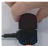
2. Move the actuator closer to the switch to start the teaching procedure. The red LED turns ON. After 10 seconds, the yellow LED gives brief cyclic flashes. Turn the power OFF. *
