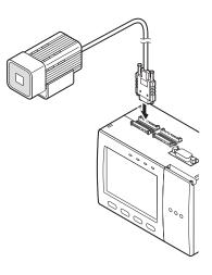
**1** Insert the camera's connector into the Controller's Camera connector.
