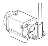
On the Controller side, the cable bends towards the rear.
