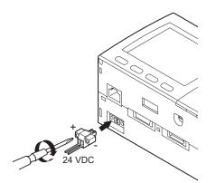
**1** Loosen the two screws on the top of the Power connector (male) using a flat-blade screwdriver.
