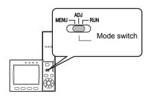
The ZFX-C has the following three modes. Switch to the desired mode before you start operation. To switch the operation mode, use the mode switch.
