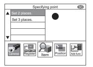
Place the measurement target at the 1st point, and select either [Set 2 places.] or [Set 3 places.].
