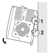
**1** Hook the Controller's upper hook onto the DIN track.
