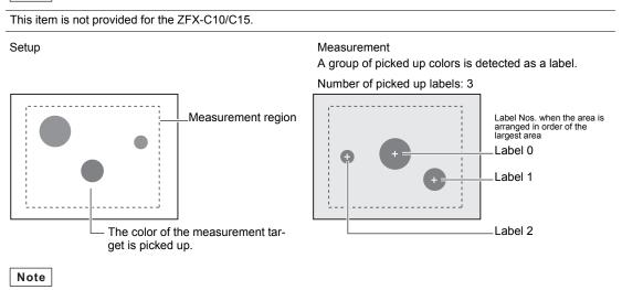
When a color camera is connected, up to four colors can be specified as the color to be measured. When a monochrome camera is connected to the Controller, black-and-white images are binarized. White pixels are targeted in measurement.
