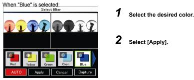
The color bar is displayed when [Custom] is selected from the color filters. You can set any color from this color bar to custom filters.
