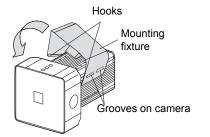
Align the two hooks on one side of the mounting fixture with the two grooves on the camera body.
