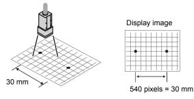
Both the origin and the coordinate system can be corrected.
