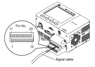
Cable diameter: 0.14 to 1 mm<sup>2</sup> (AWG26 to 16 twisted lead) Cable length: 30 m Tightening torque for the respective wire: 0.22 to 0.25 N•m Tightening torque for the Terminal Block Adapter: 0.3 N•m Terminal block adapter mounting screws: M2.6 x 7 screws (accessories, 4 p'ces)
