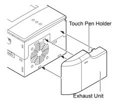
**1** Attach the Exhaust Unit to the four mounting holes on the Controller.
