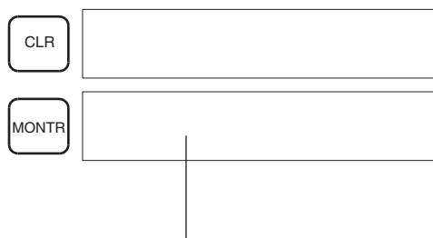
Indicates the mode set by the mode selector switch.
