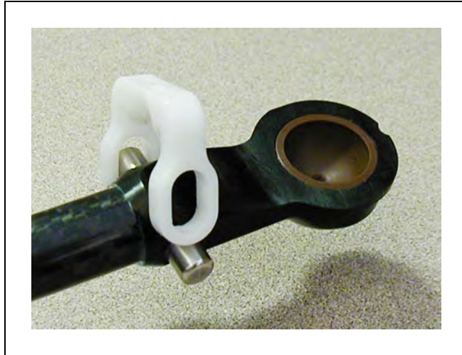
Figure 7-14. Horseshoe over One Pin
