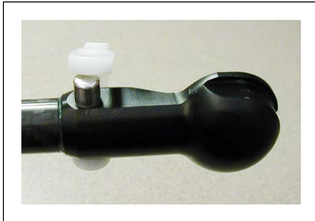
Figure 7-15. End of Horseshoe on Pin
