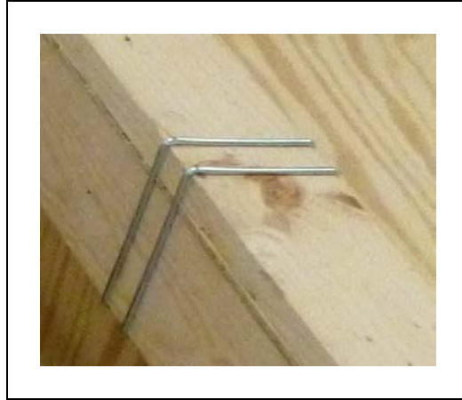
Figure 3-1. Klimp Fastener on Crate
