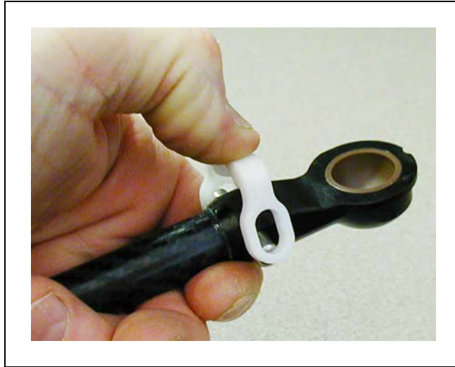
Figure 7-16. Squeezing the Horseshoe into Position
