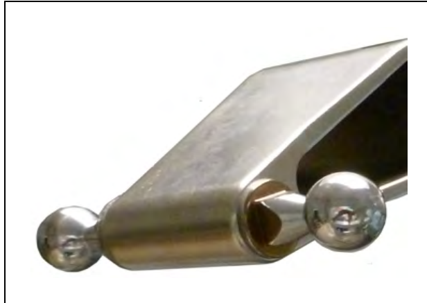
Figure 3-6. Inner Arm Ball Studs
