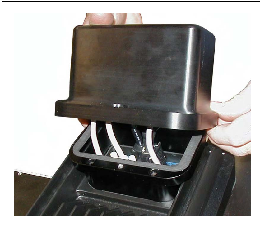
Figure 6-13. Installing Cable Entry Top Cover Assembly
