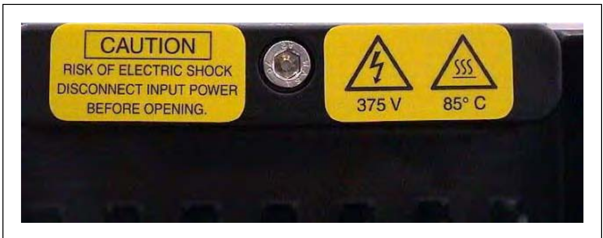
Figure 7-18. Securing Screw on eAIB Chassis
