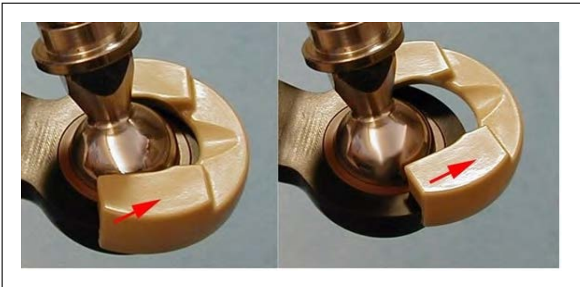
Figure 6-17. Removing a Ball Stud Lock
