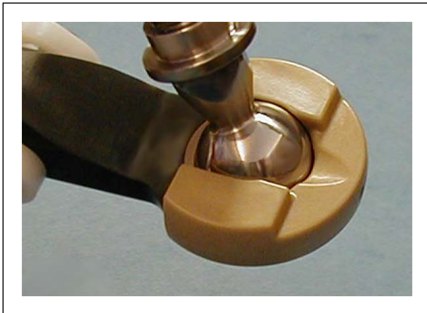
Figure 6-15. Ball Stud Lock on Ball Joint Socket
