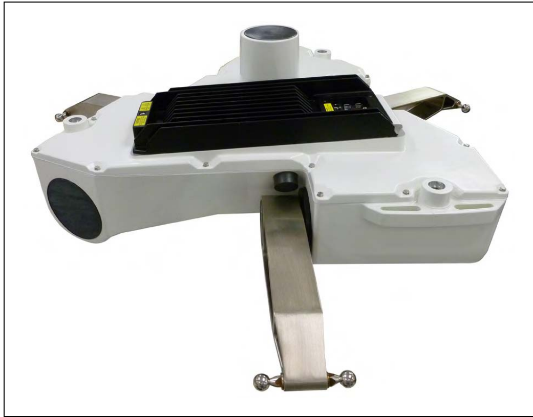
Figure 7-17. eAIB on Hornet 565 Base
