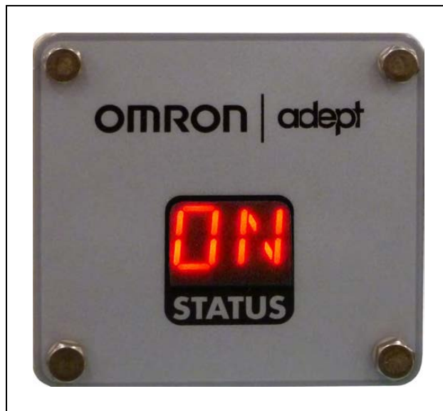
Figure 5-1. Robot Status Display Panel
