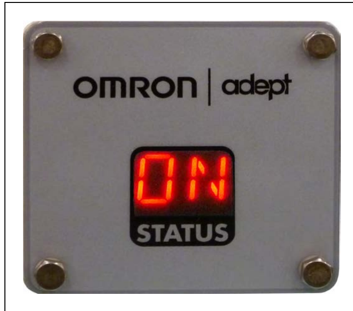
Figure 7-9. Status Display Panel Face
