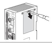
The battery is installed behind this cover.
