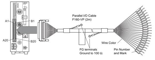
Turn OFF the power supply before connecting or disconnecting a Parallel I/O Cable. Peripheral devices may be damaged if the cable is connected or disconnected with the power ON.
