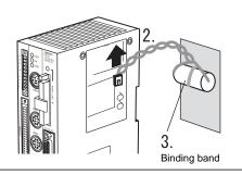
**4.** Install a new battery in the reverse order of removal. Secure the battery with the binding band supplied with the battery.
