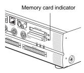
**3.** Press the eject button to the right of the Memory Card slot.
