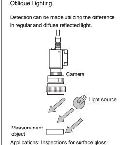
A stable image can be obtained with few shadows from uneven surfaces on the measurement object.
