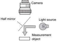
Applications: Surface inspections, positioning, and hole inspections of comparatively small objects
