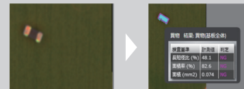
Foreign object (0402 scattered chip) detection example
