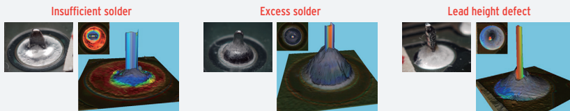
Flow solder/insertion component inspection examples
